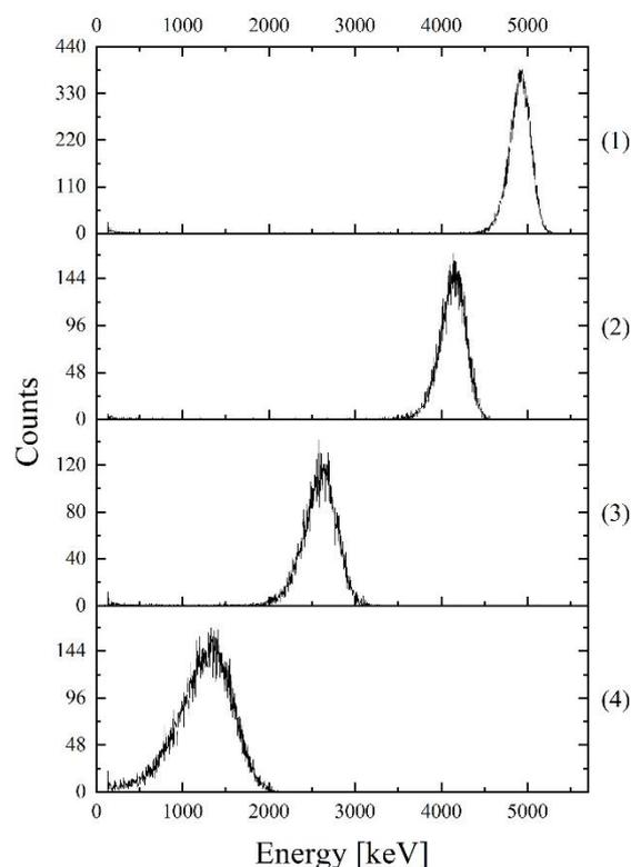
Figure 2. The measured  $\alpha$ -energy distribution functions measured by Si-detector at angle  $\theta=0^\circ$ . (1) - spectrum measured in vacuum, (2) – spectrum in vacuum after passing 6 $\mu\text{m}$  of Mylar, (3) – spectrum in air at distance from the source of 17 mm, (4) – spectrum in 17 mm of air and 6 $\mu\text{m}$  of Mylar.
