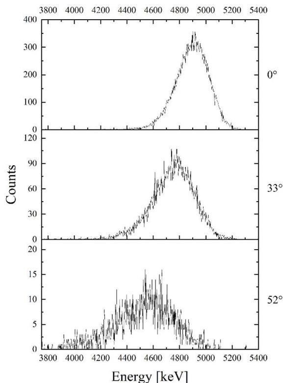
Figure 3. The energy spectrum of a flat source obtained for measurements showing different emission angles ( $\theta=0^\circ$ ,  $\theta=33^\circ$  and  $\theta=52^\circ$ )
