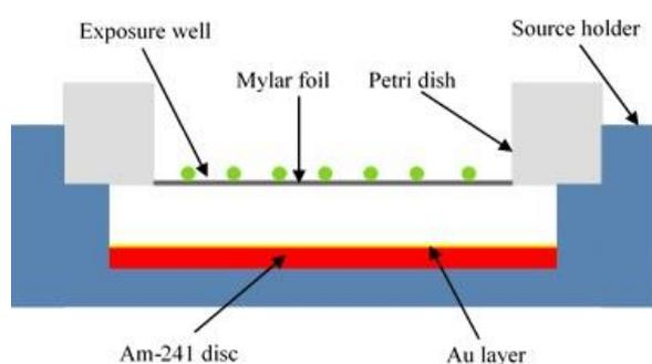
Figure 1. Schematic view of the irradiation device. The Petri dish bottom made of Mylar foil is located 5mm from the source surface. The distance between the source and Petri dish can be changed.
