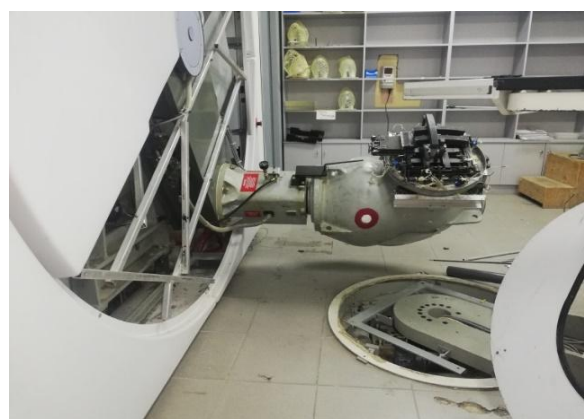
Figure 3. Dismantling process of collimator head
